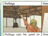
make a small force lift a heavier load. The more wheels in a pulley, the less force is needed to lift a weight.
